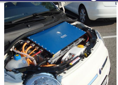
Fuel Cell system installed in electric FIAT 500
