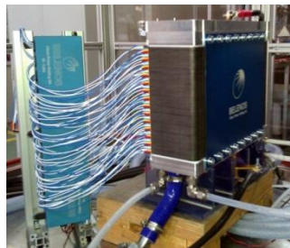
Fuel Cell stack tested at PSI
